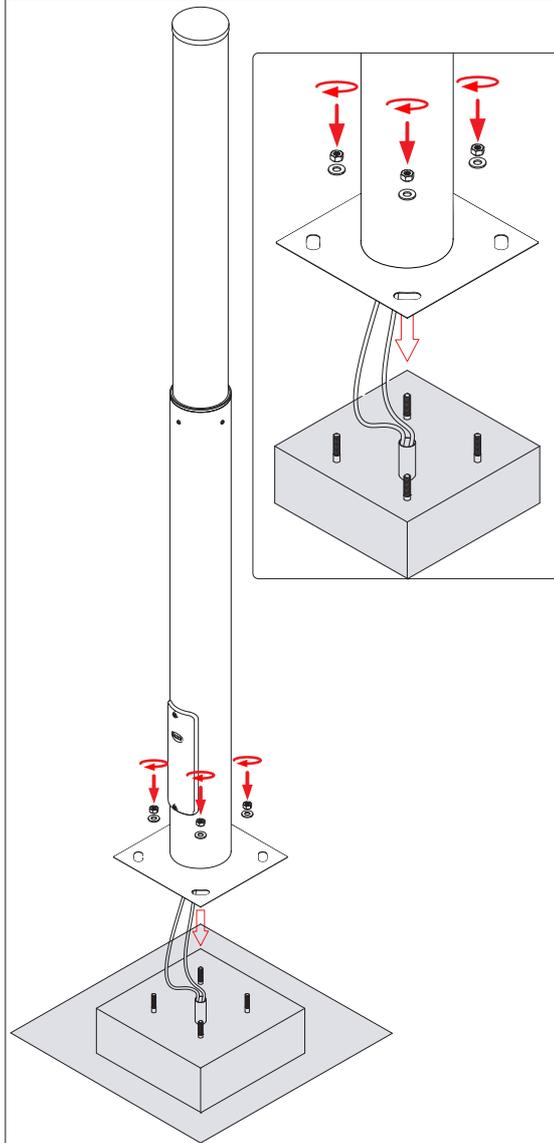
Please ensure that the wires are connected to the right polarity [Phase, Neutral & Earth]. For 3Phase Loopin Loopout connections, use appropriate Red, Yellow, Blue for Phase, Black for Neutral and Green for Earthing Terminals.
