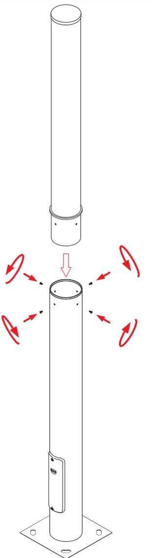
Lock and unlock the screws following an alternative sequence, tightening all screws evenly.
