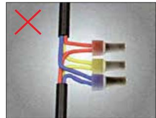
When the wire is connected into the fixture through cable gland, the cable must be more than 10mm inside. Please refer to the images below.
