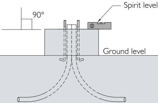
The size of the foundation depends on the topography, condition of the soil and must be determined as per site condition.
