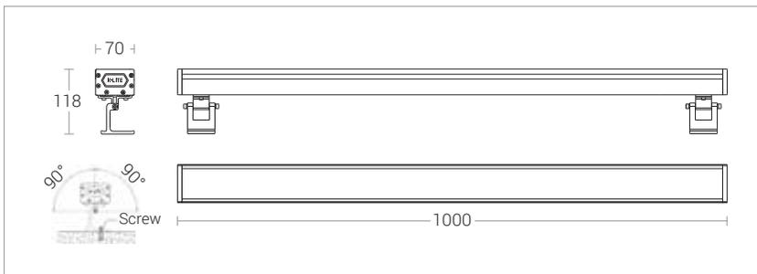
Surface mounted LED luminaires suitable for wall, ceiling & floor applications which adds elegance to commercial, historical and modern architecture.
